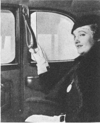
Window in new Ford opened from the front edge to permit draft-free ventilation of the interior of the car
