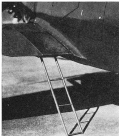
Above: The built-in passenger gang-plank on an Autogiro partly withdrawn from its housing. Below: The ladder fully extended for use
