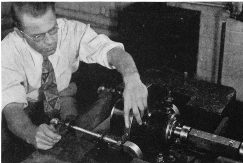
Finger points to water jet in machine for determining erosion of steel by water
