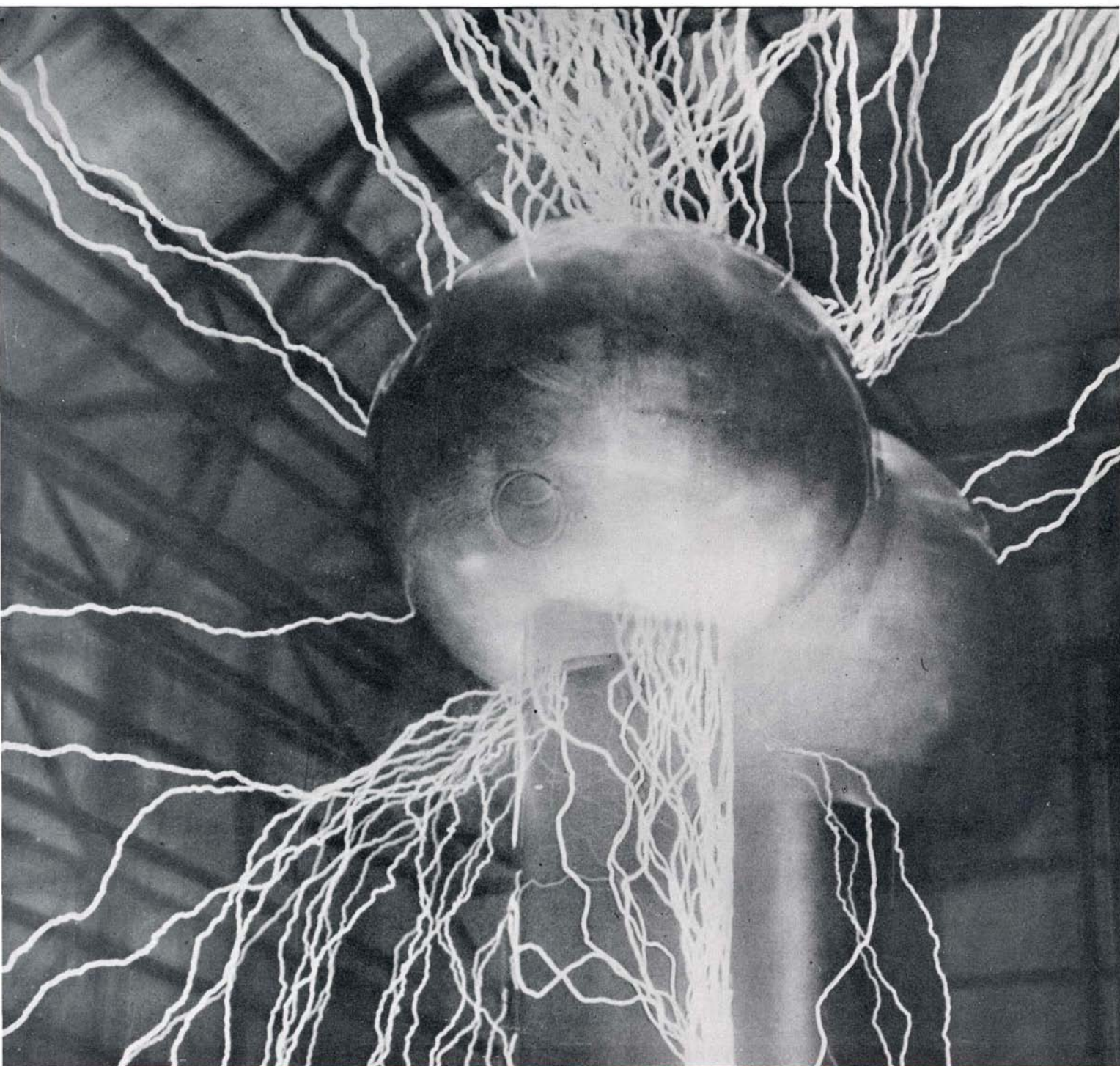
Streamers of Sparks From Van de Graaff's Generator (See page 132)
