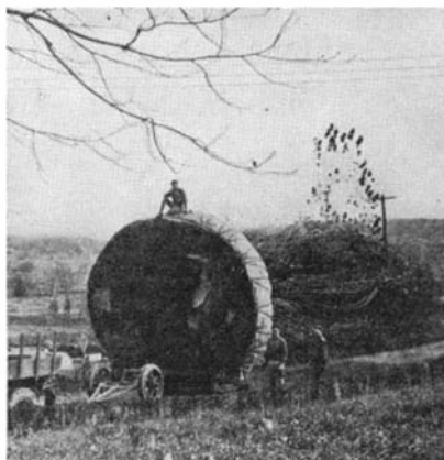
Above: A tree mover with a capacity up to 10 tons. Right: A beautiful specimen of a huge tree loaded on an arc-welded mover with a dead-weight capacity of 30 tons
