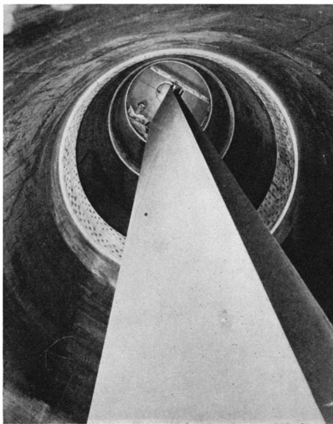
Looking up through one of the insulating columns of the Van de Graaff generator, showing the endless paper belt
