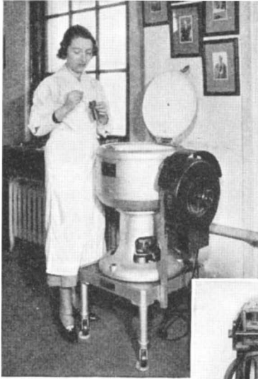
Left: Placing the tubes of blood in the centrifuge where they are rapidly whirled in order to accelerate the reaction for the M-N tests
