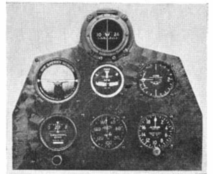
An airplane instrument board with the seven necessary instruments
