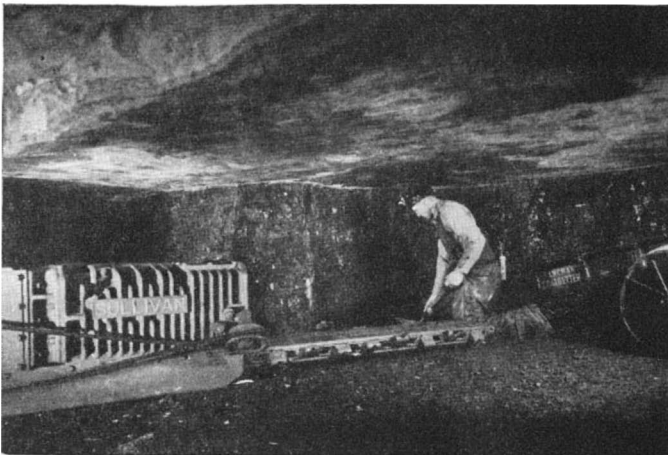
Circle: A miner, working with regular equipment, demonstrates how an undercut and shear are made
