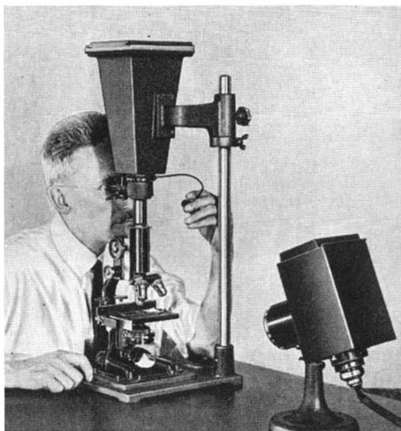
A simple type of professional photomicrographic equipment. The observation eyepiece permits the user to see the specimen till it is photographed
