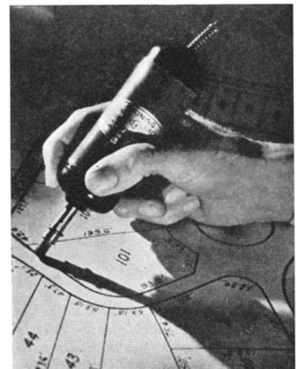
A small electric motor drives the draughtsman's high-speed eraser
