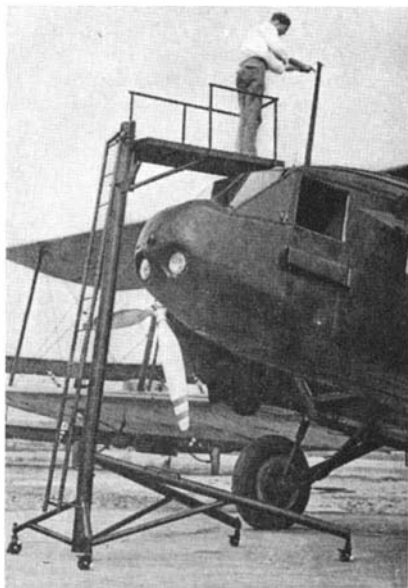
A special portable ladder used in the shops of Eastern Air Transport at Atlanta, Georgia. With this ladder it is easy to reach many out-of-the-way parts of an airplane for complete inspection or maintenance
