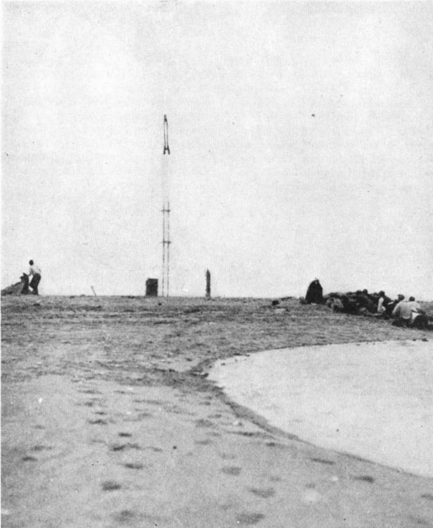
The first successful flight of a liquid fuel rocket in this country, near Staten Island. Mentioned in the text. Because of faulty design this rocket burst at an altitude of about 300 feet, after reaching a velocity of 175 feet per second
