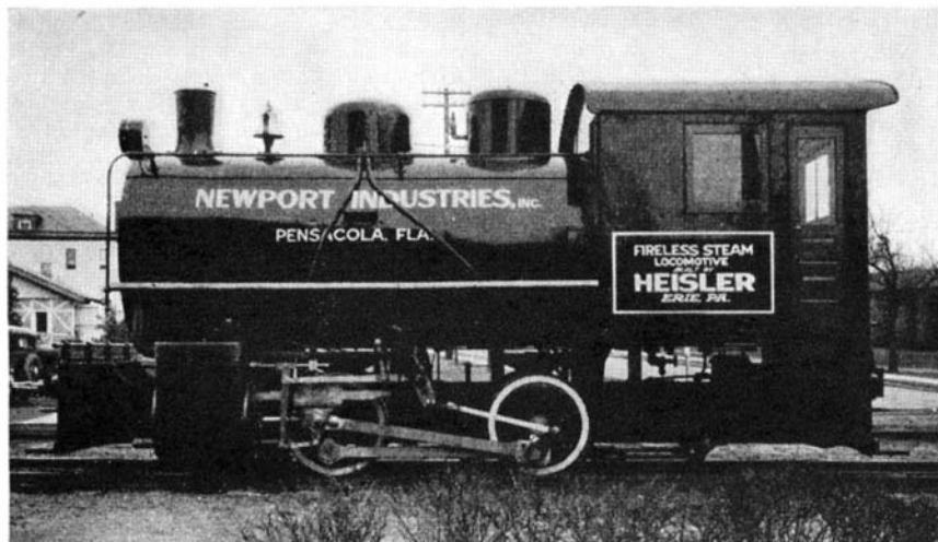
The fireless locomotive will run 95 miles on one “charge”
