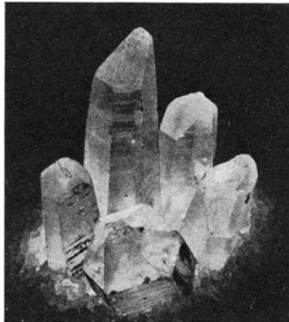
A group of quartz crystals as they are delivered to the cutters' bench
