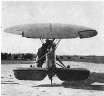
Above and right: Two views of the airplane with 15-foot circular wing
