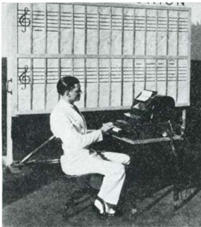
Keyboard from which chimes may be played from a far distant point
