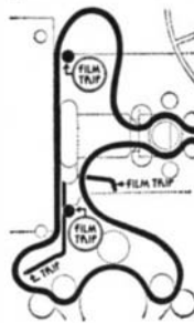
Mechanism that stops the film in a movie projector before breakage
