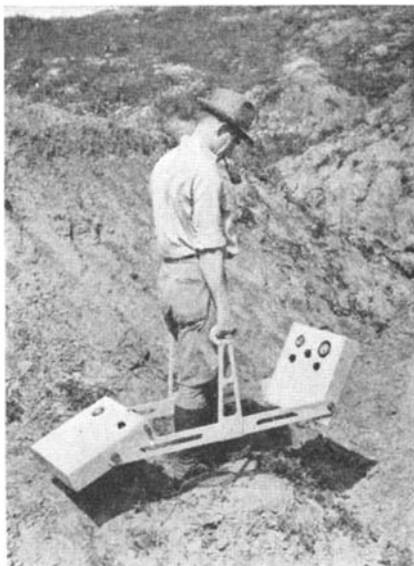
Showing how the geophysical instrument is carried when in use
