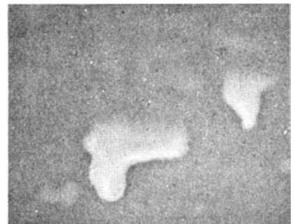
Right: An air bubble trapped on the surface of the film caused this spot. Left: Water spots on drying films are often caused by excess heat
