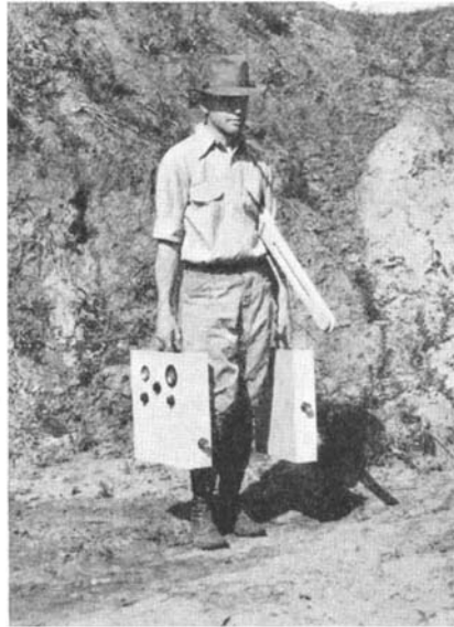
Two easily carried units constitute the geophysical instrument
