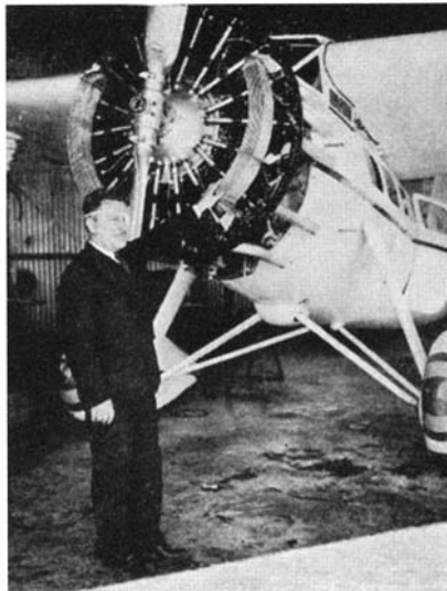
Post points to one of the radiators which are to cool supercharged air
