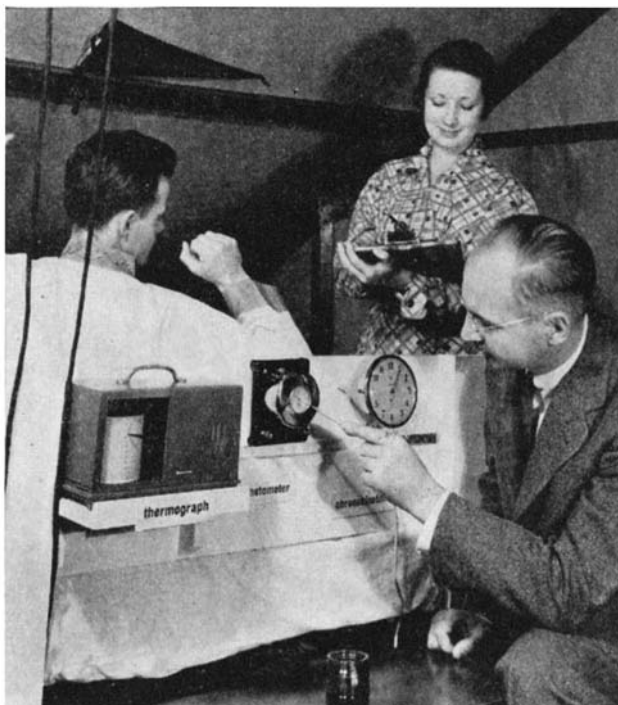
A bed in the sleep laboratory in the author's home. Thermograph at left records the temperatures. Dial of kinetometer to which Dr. Laird is pointing shows the total vertical displacement of top of mattress during the night. Special clock records all turning over in bed
