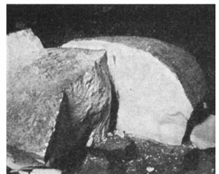
Nickle-copper block (see above) is broken by mechanical fracture
