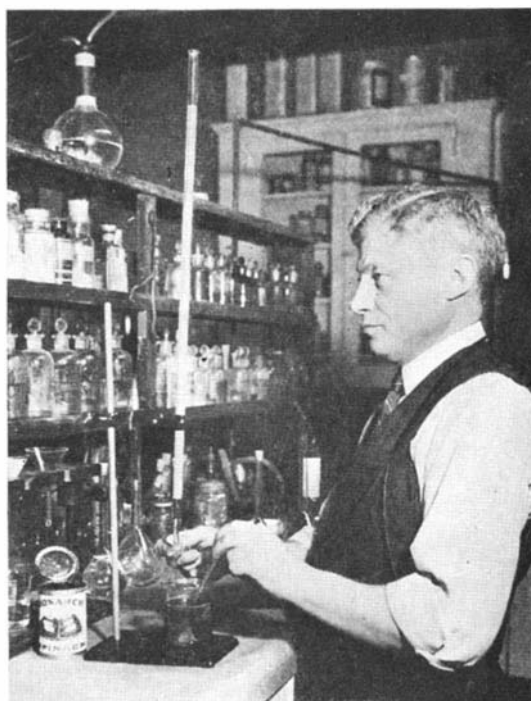
Above: At every step in the preparation of quality brands of canned foods, chemists make tests for purity. Here a laboratory test is being made to determine the acidity of one brand of canned spinach
