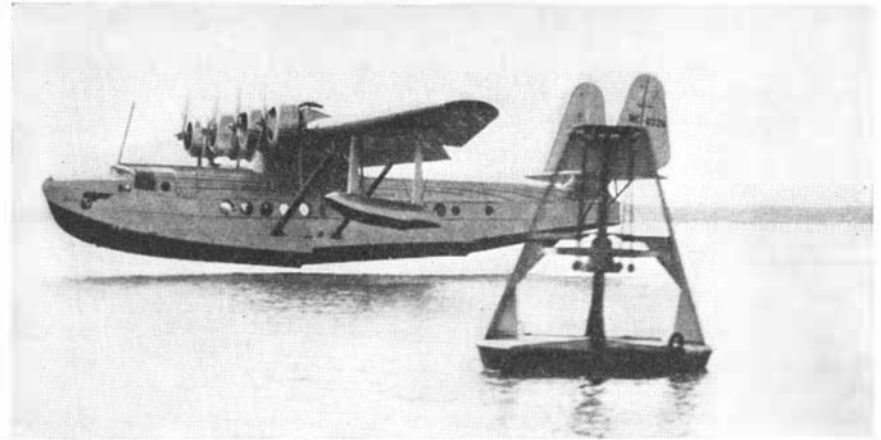
The Brazilian Clipper alighting with flaps depressed
