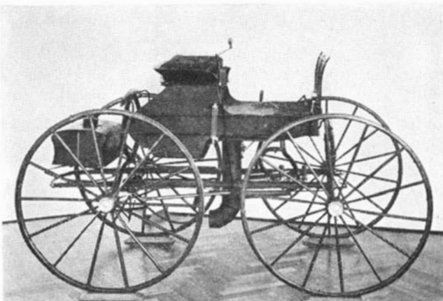
Austin—1862-63—was a steam-driven vehicle in which the power plant was located in the center under the body
