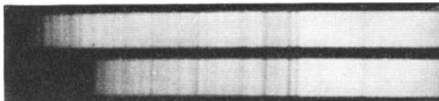
An interesting pair of spectra, not connected with Professor Russell’s present article, but reproduced because available at the time. They pertain to the new aluminized or evaporated aluminum mirrors for telescopes, which permit astronomers to photograph the spectrum considerably farther into the ultra-violet than previously. Bottom spectrum reflected from silver mirror, top one from aluminum. Both are shown cut off in middle, at the green (right end). Kindly furnished by Dr. John D. Strong, of the California Institute of Technology, who has been largely responsible for the development of the evaporation process for aluminum and other metals
