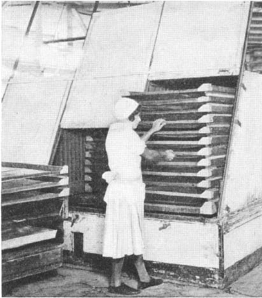
Left: To insure that dried spinach will be free from injurious properties, it is fumigated in long indoor ovens
