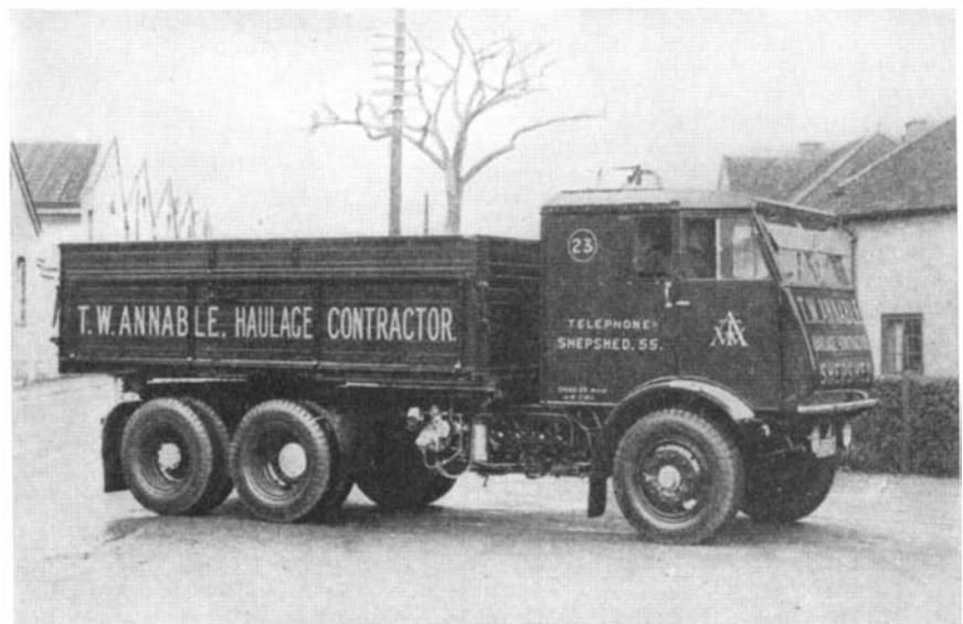
A type of coal-burning steam lorry used in England
