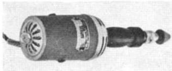
Portable grinder for small hand operations, weighing only four pounds
