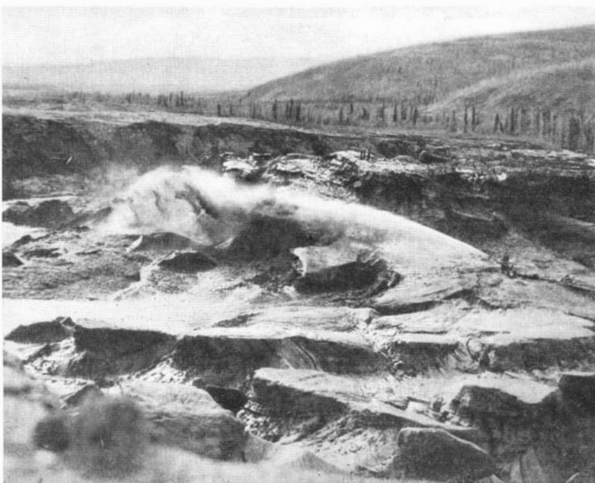
How the finds came to be exposed: Stripping off overburden with a "giant"
