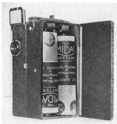
Left: Amateur movie camera-projector that uses dry cells. Above: Battery box open, showing cells. Right: Inserting the center-perforation film in the simple gate provided
