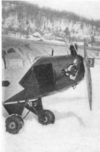
Simple yet strong engine mounting used on the Taylor "Cub" described
