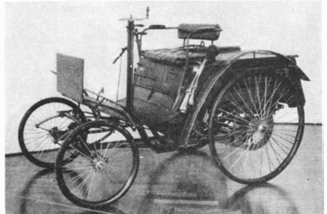
Benz Velociped—1892. Rear engine mounting. Many a sport roadster today proudly displays the same type of horn
