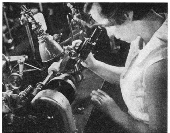
Automatic winding machines form the fine wire into coils, the operator checking the work through a microscope
