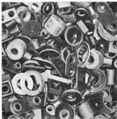
Below: Layers of fabric or paper, impregnated with plastic varnish, are pressed to yield a laminated material. Right: Some uses for this product
