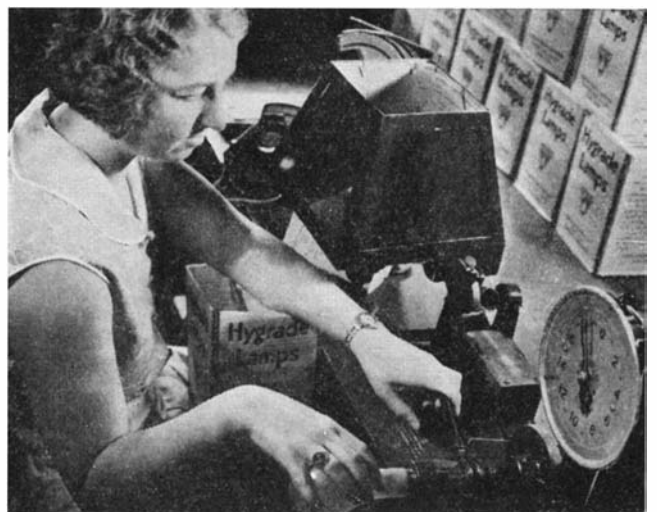
Base twisting test to determine if base is properly cemented. Scale indicates strain in pounds applied by the tester
