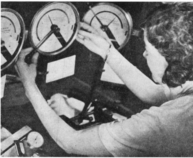
Delicate torsion balances check the diameter of filament wire before it is coiled. Eight-inch lengths are weighed
