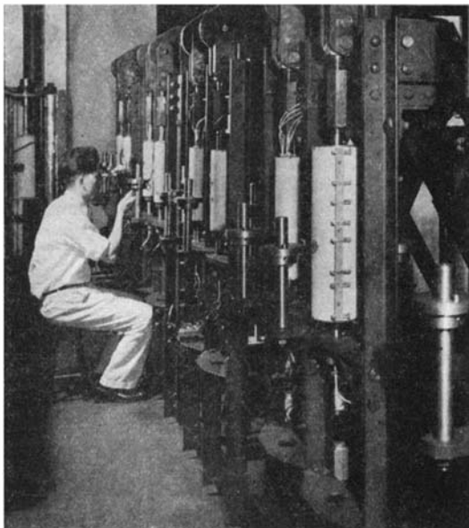
Determining elongation in a number of creep tests of steel. Telescope micrometer is used
