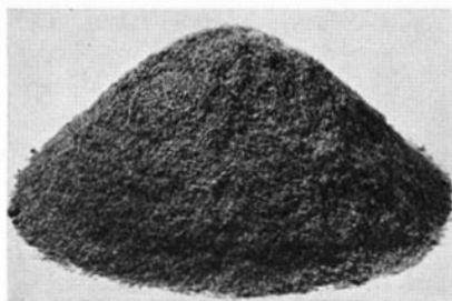
Above: Making phenolic objects in a multiple die under hydraulic pressure. Left: A pile of the raw material from which such objects are molded
