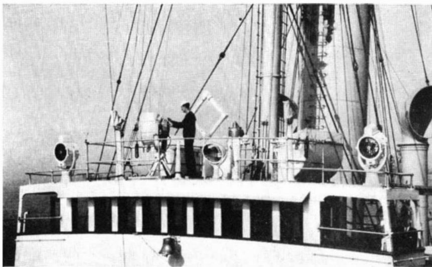
The high-power loud speaker mounted on the bridge of the Tampa
