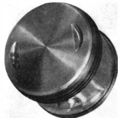
The heads of the pistons in the new Wasp engine are flat, but recesses have to be provided for the valves
