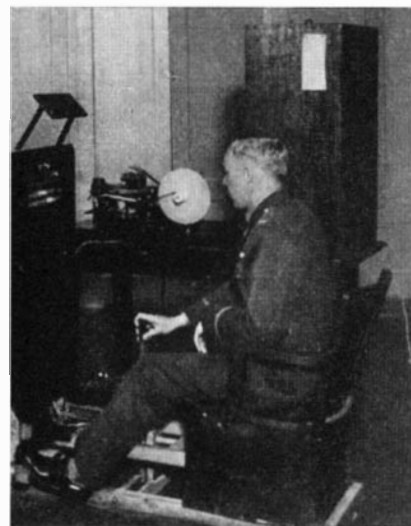
A pilot's flying ability is checked by the use of this co-ordinator
