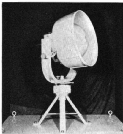
The 500-watt loud speaker or "bull-horn" to replace the megaphone
