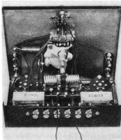
Left: A five-meter transceiver in use. The long tubing is the antenna. Above: The interior of the unit, showing its extreme compactness
