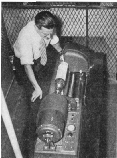
Wirephoto transmitter: A picture is in place on the scanning drum
