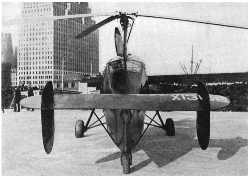
Rear view of wingless Autogiro, showing steerable tail wheel
