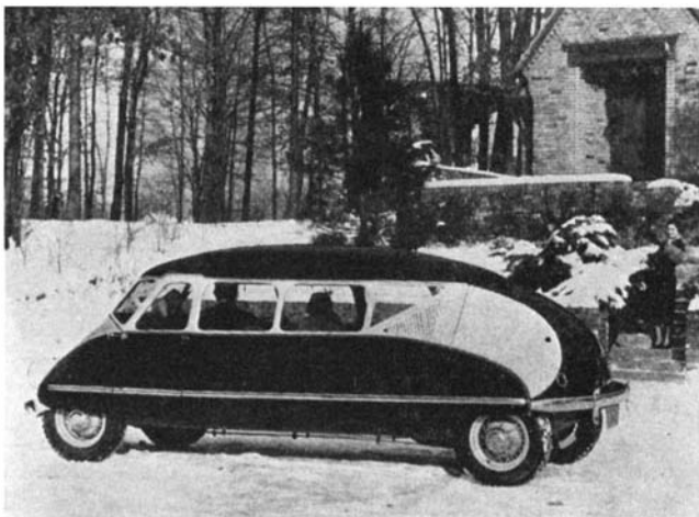
The new Stout "Scarab" motor car with rear engine mounting and a body designed to facilitate easy steering
