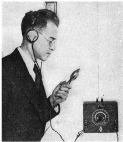
Left: A five-meter transceiver in use. The long tubing is the antenna. Above: The interior of the unit, showing its extreme compactness
