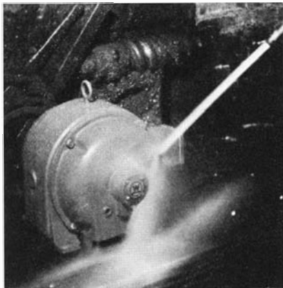
A stream of water from a hose fails to penetrate this water-proof motor
