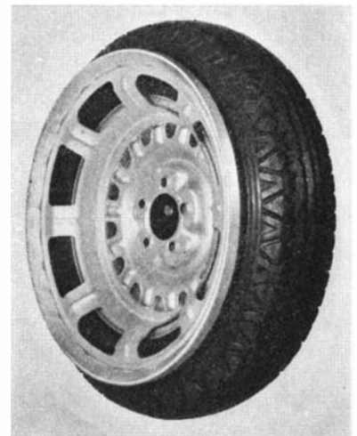
The Tire Guard, showing how it is rigidly attached to the car wheel
