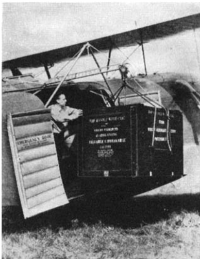
Monorail hoist with which large cases can be loaded into the Condor
