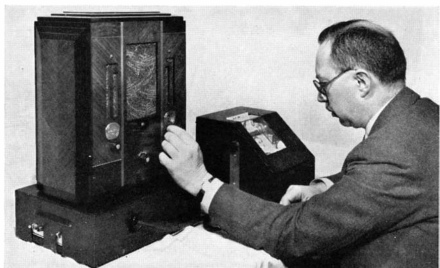
A facsimile receiver coupled to an ordinary type of home radio set
