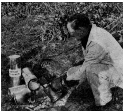
Heating Nitramon with a blow torch to demonstrate safety of explosive
