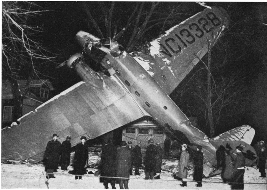
Structural strength of transport planes plays an important part in air safety. In this crash, the entire passenger cabin remained intact; only the pilot and co-pilot were slightly injured
