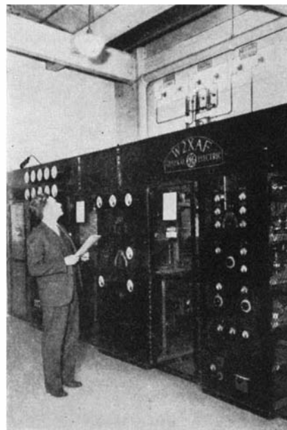
W2XAF, Schenectady, New York. Antenna wave-change switch at top
