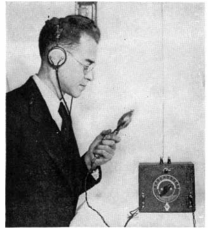
Above: A five-meter transceiver in use. The long tubing is the antenna. Below: The interior of the unit
