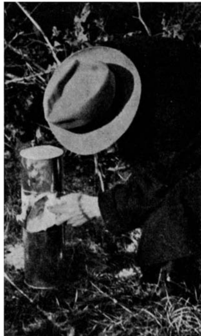
A rifle bullet tore through the Nitramon but did not detonate it
