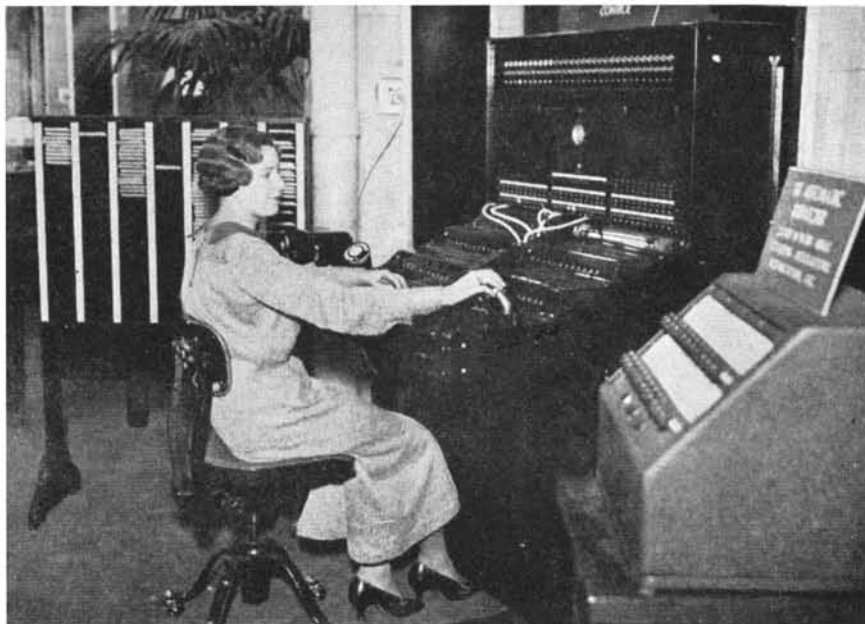
No, the young lady is not playing a pipe organ, nor is she operating a telephone switchboard. She is demonstrating a model factory production control system introduced by Remington Rand. By means of this, it is possible for one girl to keep accurate records which now require the work of scores of time-keepers and clerks. At right is the automatic punch which produces the basic record
