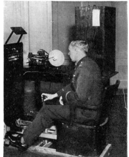
A pilot's flying ability is checked by the use of this co-ordinator
