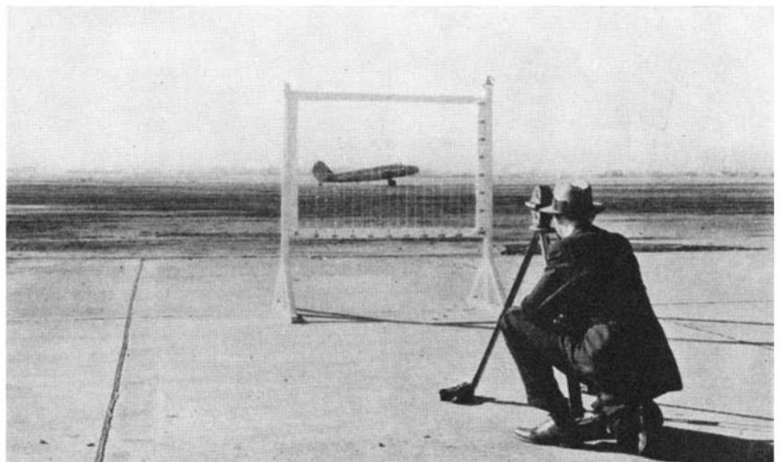
How a camera is applied to the job of measuring airplane landing speed
