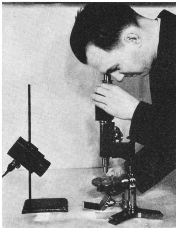
Figure 6: The polarizing apparatus in use. Mica plate is being held below the microscope stage
