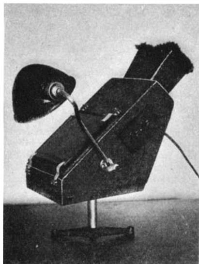
New laboratory cabinet for use in examining fluorescent substances
