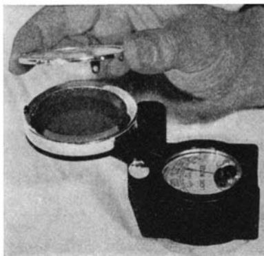
A screen for light meters that multiplies the range to 10 times normal
