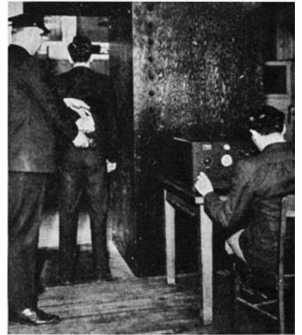
The parallel loops of the gun detector are concealed in the door frame
