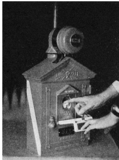
An alarm that prevents false alarms; warning bell mounted above fire box
