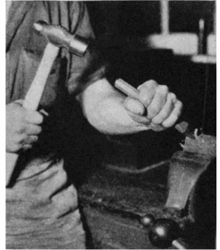
A cold chisel, tipped with a copper alloy, cuts a cold rolled steel bar
