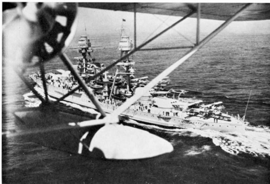
The U. S. S. Pennsylvania , flagship of the United States Fleet. This aerial photograph shows four planes and two catapults, also the hull's blister protection
