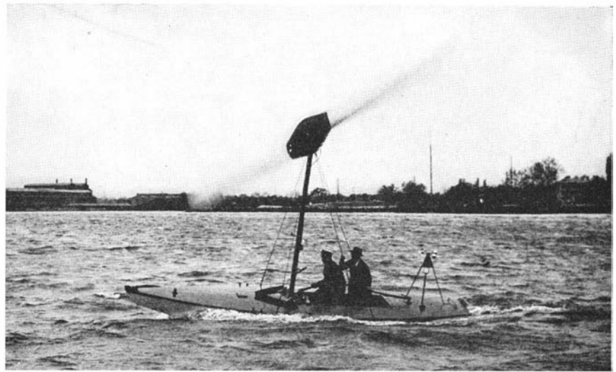
The mast of the gyroplane sailboat is rotated by a simple control
