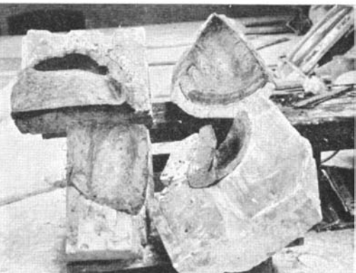
Fifth Step. Sections of glue-lined mold
