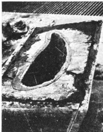
Sixth Step. Plaster mold with glue and wax shells re-assembled for making the plaster core
