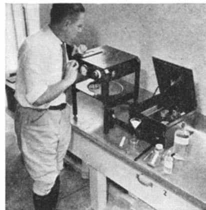
The rotating part of the soil analyzer is in a shelf directly below the cabinet containing the light source
