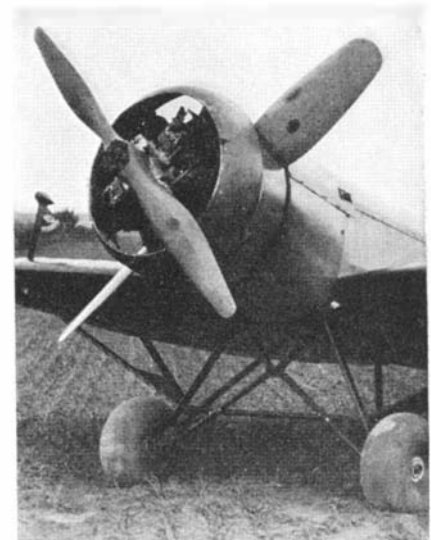
How the engine and two propellers are arranged for anti-torque drive
