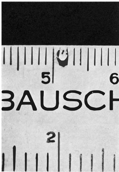
Figure 5: A tiny lens, worked to a precision of a millionth inch
