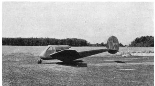
Side of the Hammond plane, showing the three-wheel landing gear, the attitude of ship at rest, and the booms
