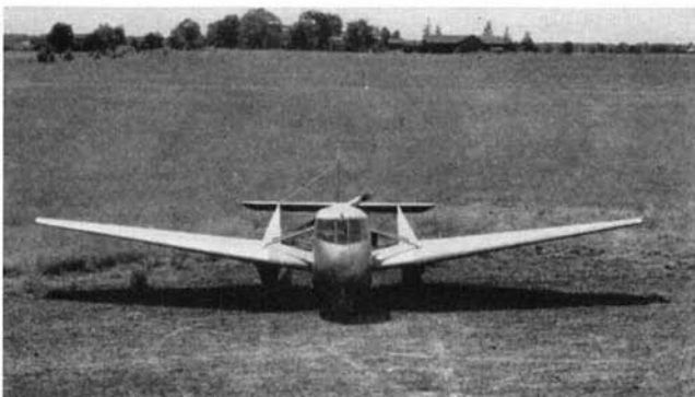
Front of the Hammond pusher, described above, powered with a Menasco four-cylinder, in-line, air-cooled engine
