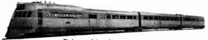
Below: 3600 h.p. Winton-Diesel passenger locomotive recently placed in service to pull famous Santa Fe train, the Super Chief
