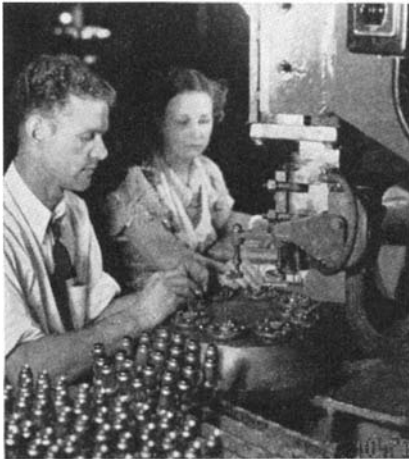
Courtesy RCA Manufacturing Co., Inc. Welding metal tube parts. In this powerful machine, Thyatron-timed currents on the order of 75,000 amperes weld the parts to form the air-tight containers for the units
