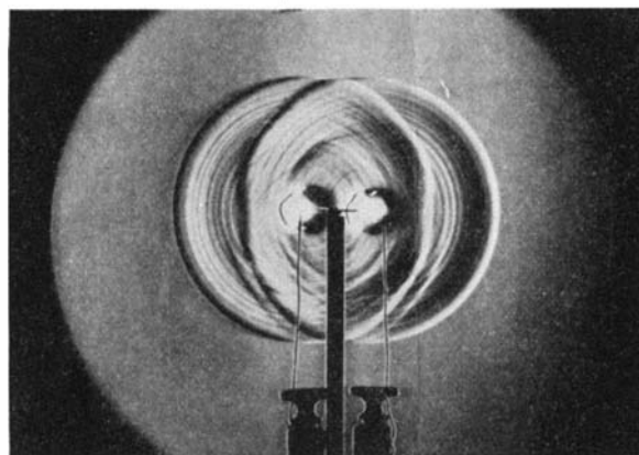
Two sound waves spreading simultaneously, and practically independently, from two spark gaps.
