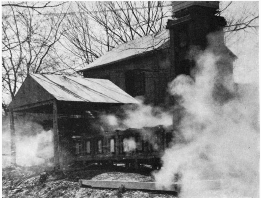
Above: An experimental dust explosion in the testing station at Arlington, Virginia. Note flying glass. Adequate venting area has prevented damage to the structure. Below: A modern grain elevator showing application of glass vents
