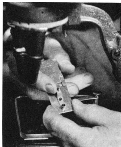
Forcing out a small part of fiber, about 2.5 microns thick, for slicing
