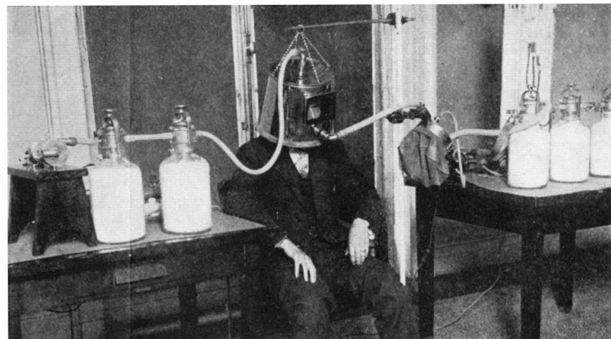
A helmet invented by Prof. Frances G. Benedict to be used for studying the chemistry of breathing. Oxygen "credit" is of very great importance to athletes
