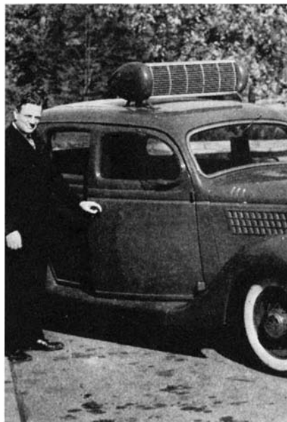
Above: Air conditioning for a standard motor car. Right: Bus equipment. A is the compressor, B the cooling coil provided with a filter, C the fan, D the distribution ducts, and E the condenser cooling coil that dissipates heat extracted from the interior of the vehicle
