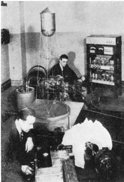
The laboratory earthquake equipment set up to test a model tank
