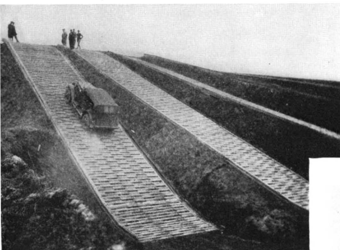
Scout cars must be tough—and powerful. This one climbed a 60 percent grade, the steepest on the slope course
