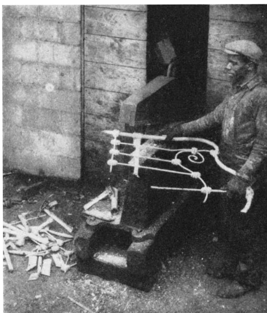
Powerful shears for cutting up metal scrap
