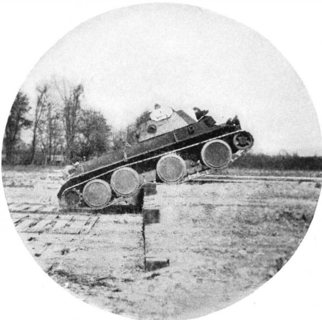
A medium tank, of the high-speed type, climbs a three-foot vertical wall, putting great strain on its track
