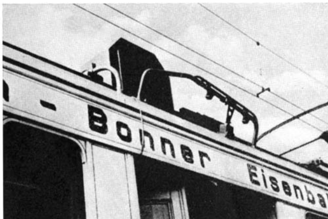
Two views of the automatic train stop, showing the tripbar on the locomotive, and the signal-post arm
