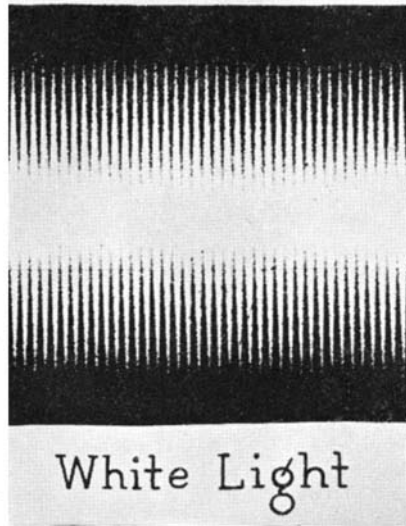
Compare photographic quality of these sound records as recorded on film by white and ultra-violet light
