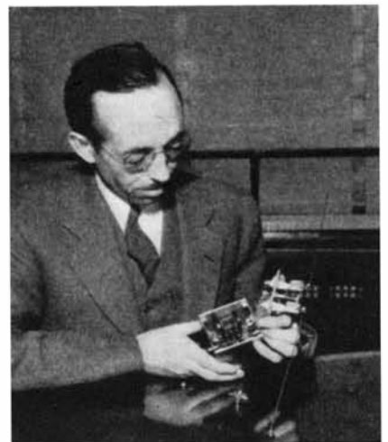
The smallest micro-wave transmitter, showing the two-rod antenna
