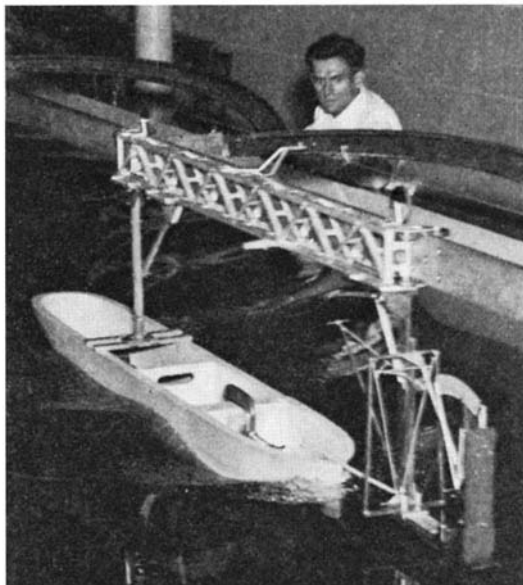
Testing a model of a Hog Island type of ship in the tank. Note bow waves and instruments
