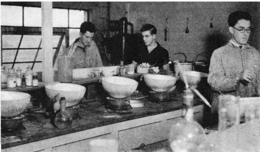
Refined work in the radium laboratory at the Port Hope radium plant, showing how the ore is reduced to a fraction of a gram for medical purposes
