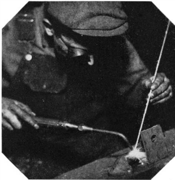
Flame welding, as an efficient mender-of-metals, quickly repairs broken machine parts of all kinds
