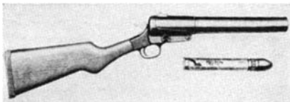
Above: Gas gun and cartridge. Below: Projectile that is made gas-tight by electric-furnace brazing
