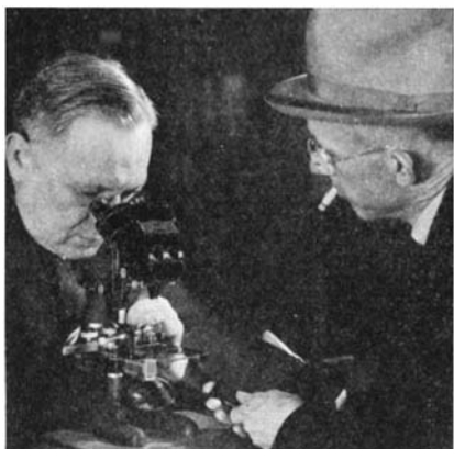
Wide-field binocular microscope fitted for examination of gems
