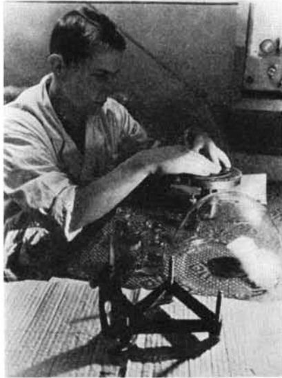
A Science Service photograph of Leonid Surodeikin, worker at the Leningrad Optical Institute, U. S. S. R., preparing equipment to be used in the July eclipse. Data about the job being done are not given, but a thin glass disk is obviously being polished on a typical pitch lap
