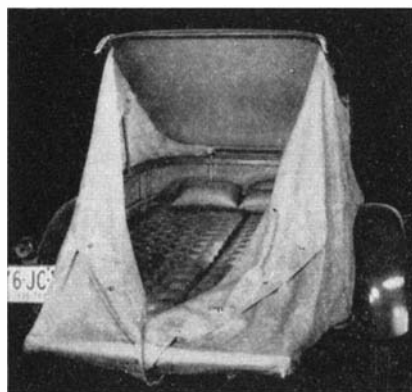
Left: A new pressed steel trailer for motor cars. Above: The trailer cover opened, showing how it may be fitted with two beds for camping
