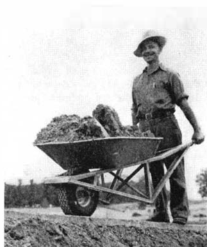
Even the wheelbarrow has been improved. The one shown is made of aluminum alloy and equipped with a rubber tire. The four and a half cubic foot size weighs 36 pounds
