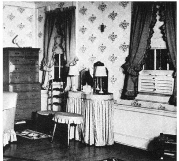
A unit for conditioning the air of a single room. This small, compact type, similar to several produced by different companies, is simple in operation, needs little attention
