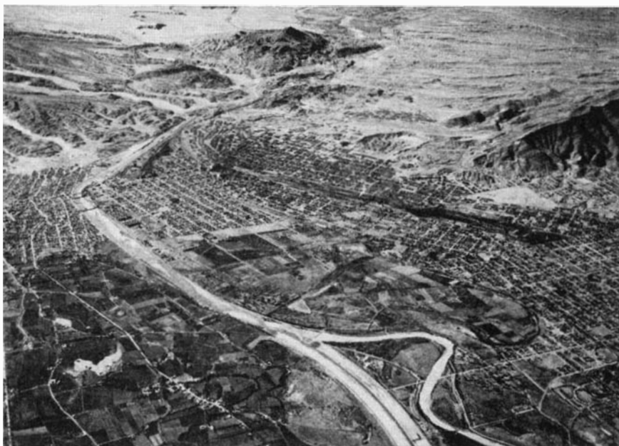
El Paso, Texas, and Juarez, Mexico, showing a portion of the new river channel. The limited work here has already improved seepage conditions in these towns
