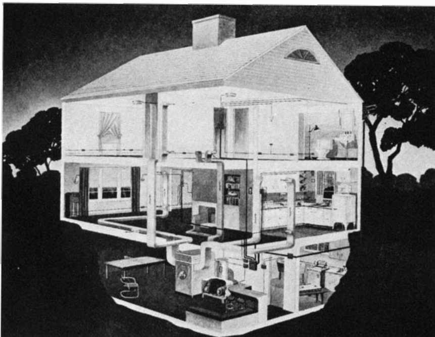
Skeletonized house showing a typical air conditioning installation. From basement units, fully conditioned air is distributed through ducts, summer and winter
