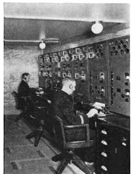
International marine radio operators in the control room on the Queen Mary . The transmitter, 400 feet away, is started or stopped from this room by a dialing system
