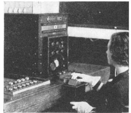
Electrical testing of bearing balls
