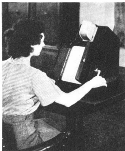
The film's tiny "pages" are projected on the screen of this device
