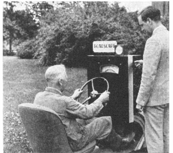
Steering skill test. Subject must manipulate the steering wheel to hold the miniature "road"
