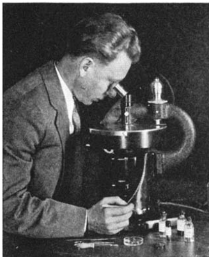
Centrifuge-microscope that proved epheogenesis possible in nature
