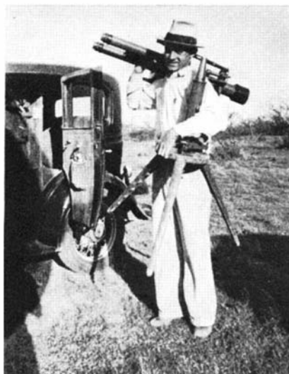
Figure 7: Returning after taking a field reading on a torsion balance
