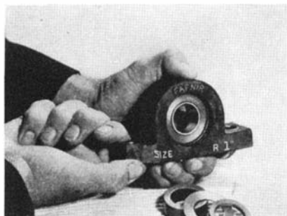
Rubber cushions a shaft bearing
