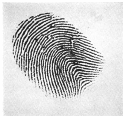
Blowing iodine fumes against a finger print on a paper surface. Dr. John McMorris looks on. At right: A finger print "raised" from a mahogany surface by the use of this method
