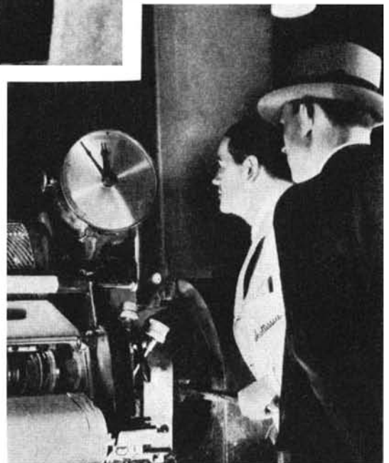
Mechanical counting of sheets of toilet paper, perforated and packed on the roll at lower left
