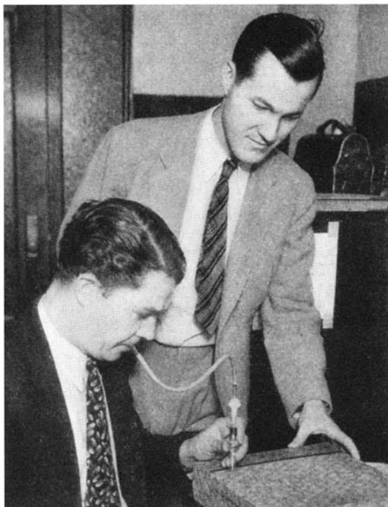
Blowing iodine fumes against a finger print on a paper surface. Dr. John McMorris looks on. At right: A finger print "raised" from a mahogany surface by the use of this method
