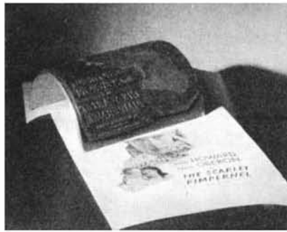
A curved synthetic rubber printing plate, and an example of its work
