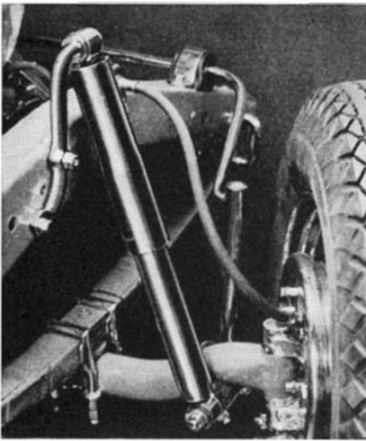
Typical of new telescoping shock absorbers is that used by Dodge
