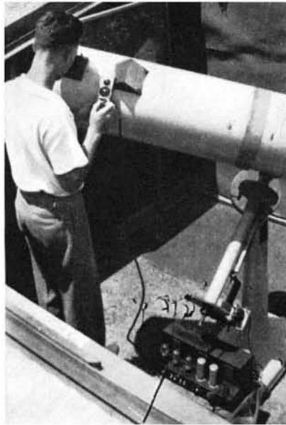
Figure 4: Using remote control to regulate the speed of the telescope
