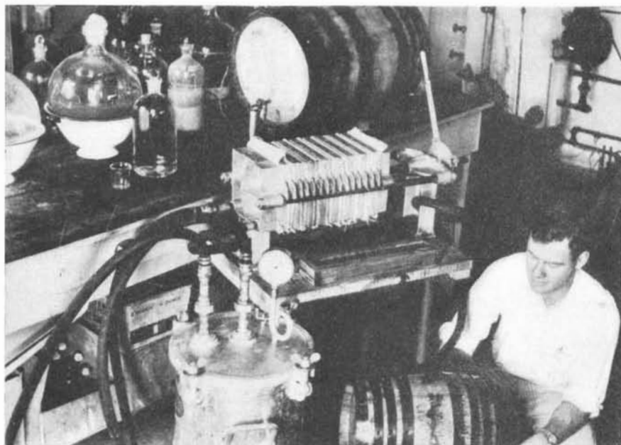
Aluminum press used in the initial filtration of citrus wines
