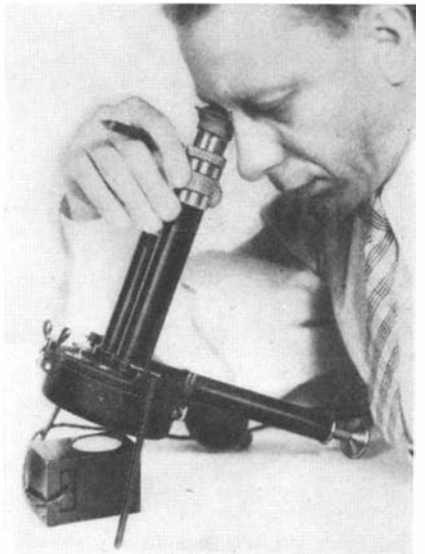
The dust counter equipment complete with its carrying case. Below: Using the dark-field microscope viewing-and-counting system. Note the sampling pump
