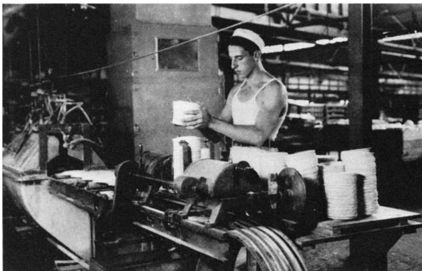
Dishes passing through the electrostatic precipitator one at a time
