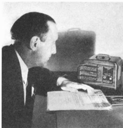
Using "Carrier Call," a telephone service on the electric light line. Below: Close-up of the combination transmitting and receiving unit
