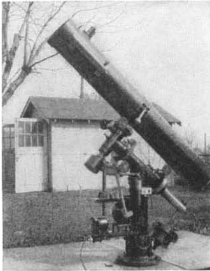
Figure 6: A sturdy and rugged mounting, made by James E. Myers, 1519 Olin Avenue, Omaha, Nebraska. The drive is of special interest (the extra "shaft" is only a pipe in the fence in the rear)
