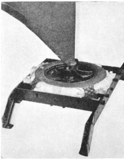
In this unique tourist trailer coupling, the road shocks are absorbed by a pneumatic casing held by an aluminum frame which is fastened rigidly to the chassis of the tow car. The nose of the trailer pivots on the center of the casing spider, with the weight thrown just forward of the rear axle of the towing automobile
