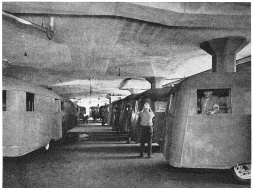
Coach trailers in all stages of assembly in a modern trailer factory
