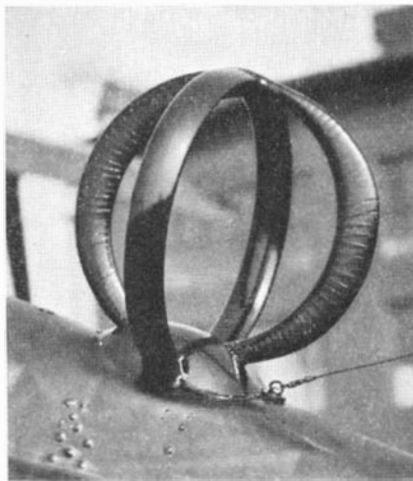
Above: The fixed loops of the Dane visual radio direction finder. Below: The rest of the equipment, with the remote control on the left and the indicating head at the extreme right
