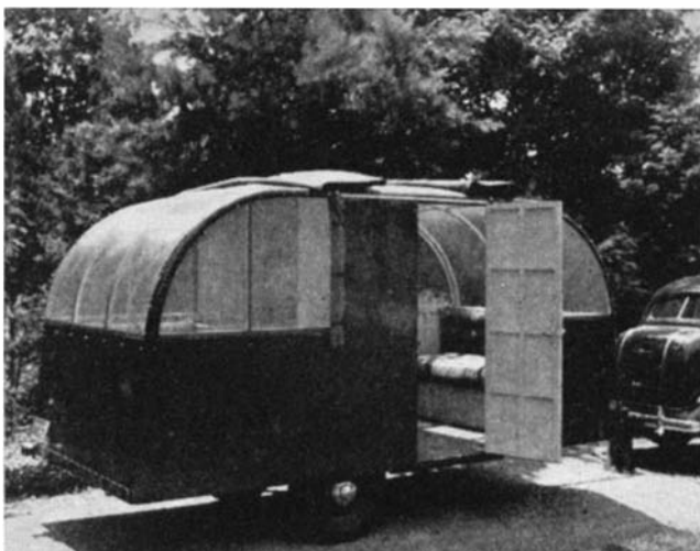
Essentially for vacation tourists, this trailer uses a combination of metal and fabric in its structure for light weight
