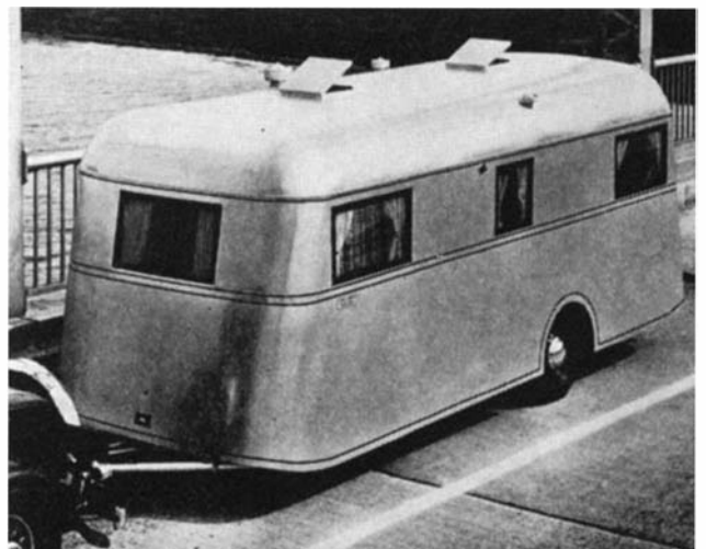
A year-'round home on wheels with heat- and sound-insulated panels of aluminum riveted to a metal frame
