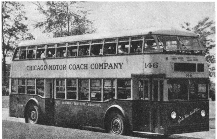
An ultra-modern coach, seating 72 passengers, with the engine mounted in the rear, and, above, a view of the upper deck, showing the seating arrangement
