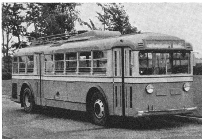
One of the "all-service" coaches pioneered by Public Service Coordinated Transport of New Jersey. These vehicles are equipped with both gasoline and electric motors and can be run either on a double-wire trolley system or under gasoline engine power on any highway, making for flexible service
