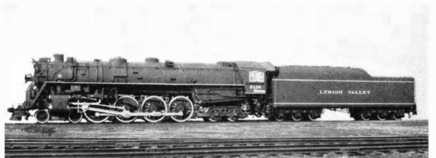
A typical modern engine built by the Baldwin Locomotive Works for the Lehigh Valley. Cylinders are 27 by 30 inches; steam pressure, 275 pounds; tractive force, 66,500 pounds; and weight, 435,000 pounds. Roller bearings are on the axles
