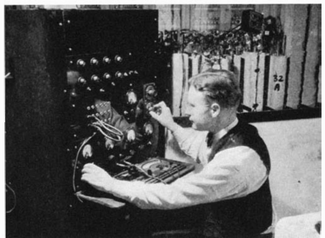
Tanks for testing concrete with sea water, and, right, the instrument board of the equipment
