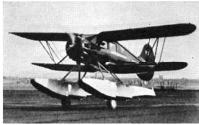
A standard Waco biplane fitted with the amphibious float gear described
