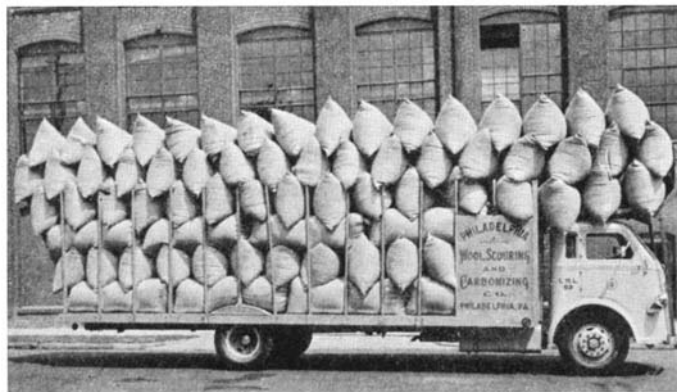
With its engine placed under the driver's cab, this 215-inch wheelbase, stake-body motor truck carries 107 bags of wool
