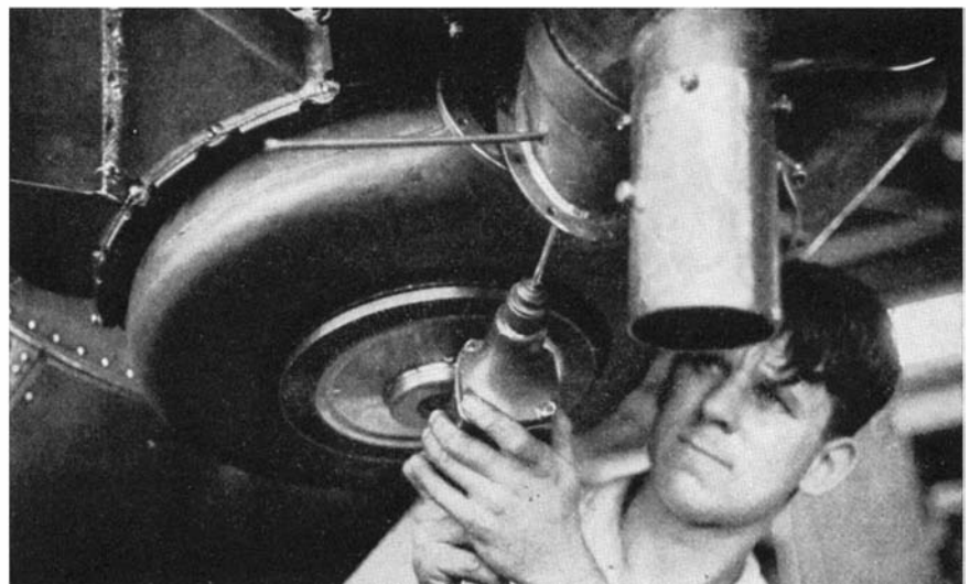
The rotor (background) of this "turbo" supercharger makes 30,000 revolutions per minute at full speed. It maintains the full engine power up to 30,000 feet
