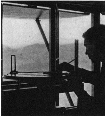
The Osborne fire finder in use to locate exactly the position of a fire. This information is then transmitted at once to the Forest Rangers
