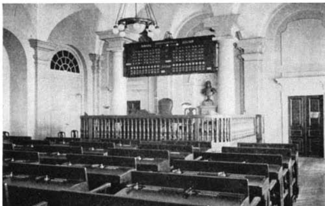
Mechanical bidding in a stock exchange. Left: The board on which bids appear. Right: The members' push buttons
