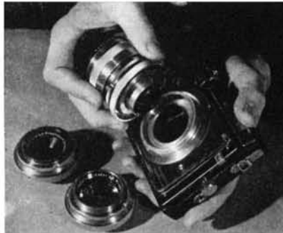
Makina II S lenses have the advantage of a “half screw” arrangement
