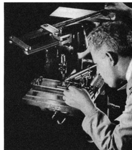
Above: The machine with which extremely fine engraving is done. Below: Enlargement of engraving in a .005 inch circle. At left: Close-up view of the engraving point and the microscope through which the progress of the work is followed
