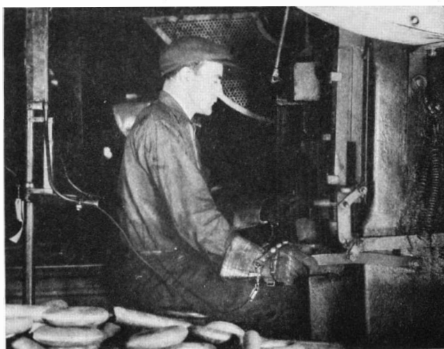
Automatic vigilance. This press operator wears wristlets; cords attached jerk his hands back if he negligently leaves either of his hands in the path of the descending punch.
