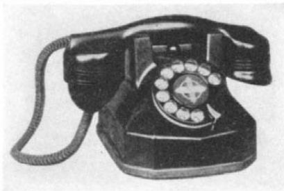
Kinkless 'phone cord in use, and, at left, in its normal shortened form
