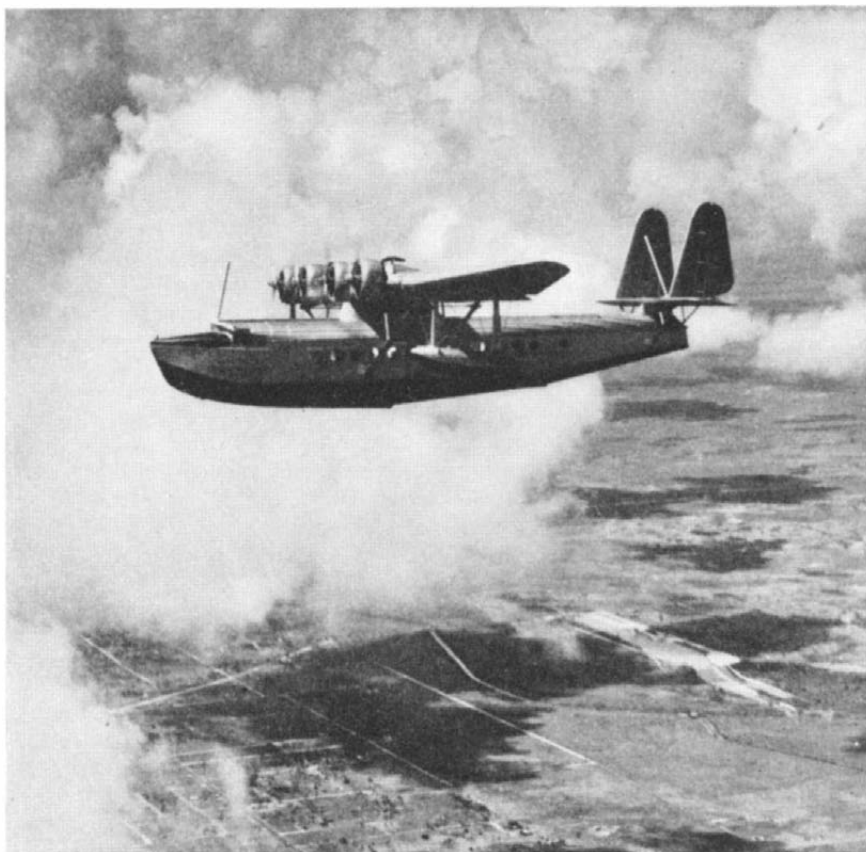
Above: Sikorsky Clipper Ship built for Pan American Airways. It is equipped with constant-speed propellers and Hornet engines, two views of which are at left and below
