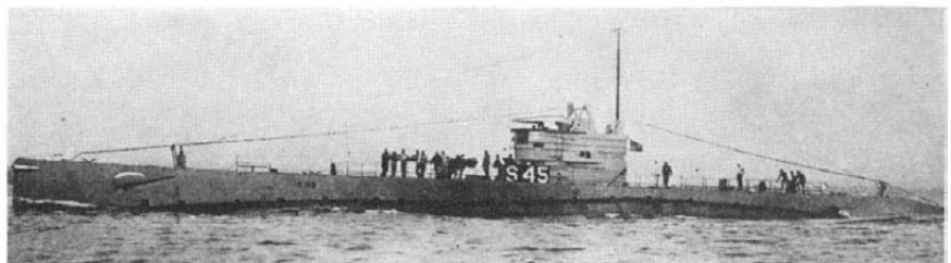
Our Navy has 45 submarines of this S-45 type, though some are smaller. She is of 850 tons (surface), carries one 4-inch gun, and has four 21-inch tubes
