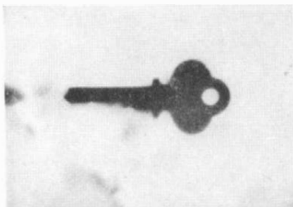
Radiograph of a key, taken with a rich piece of carnotite, an ore of radium. This is about what happened in Becquerel's laboratory
