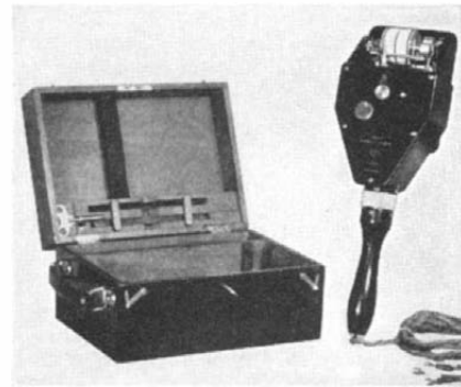
Above: The portable vibrograph, and, below, a record of vibration made by a stylus on moving celluloid
