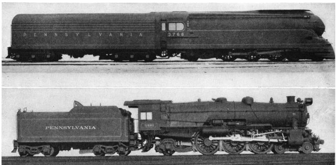
In the newer concept of railroading, streamlining plays an important rôle for operating efficiency, but also for the sake of appearance. Here we see a "before and after" of a steam locomotive. The fin above smoke stack deflects smoke
