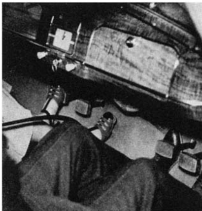
Two sets of clutch and brake pedals are used for driving instruction
