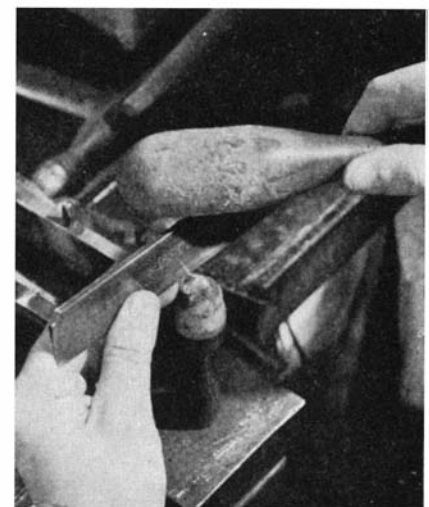
Left above: Marking cleavage lines on the rough Jonker diamond. Above: The 12 diamonds, weighing 375 carats total, that were cut from the Jonker. Right: Cleaving a piece of the diamond with a sharp blow
