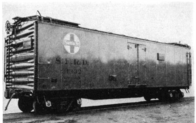
A rebuilt refrigerator car with a modern, steel superstructure and many other improvements, as described in the text
