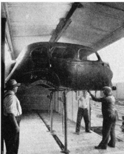
More automobile bodies per car by new loading system. Left: Automobile body on stanchions ready to be turned into place. Right: Body turned and fastened for shipment
