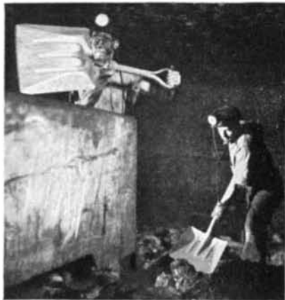
Coal miners, moving from 15 to 25 tons of coal in a day, perform a lot of work on their shovels alone. If these implements can be made lighter, yet able to stand the gaff, the miners can conserve energy. Thus the aluminum shovels, shown in the illustration above, which weigh two pounds less than ordinary coal shovels made of sheet iron
