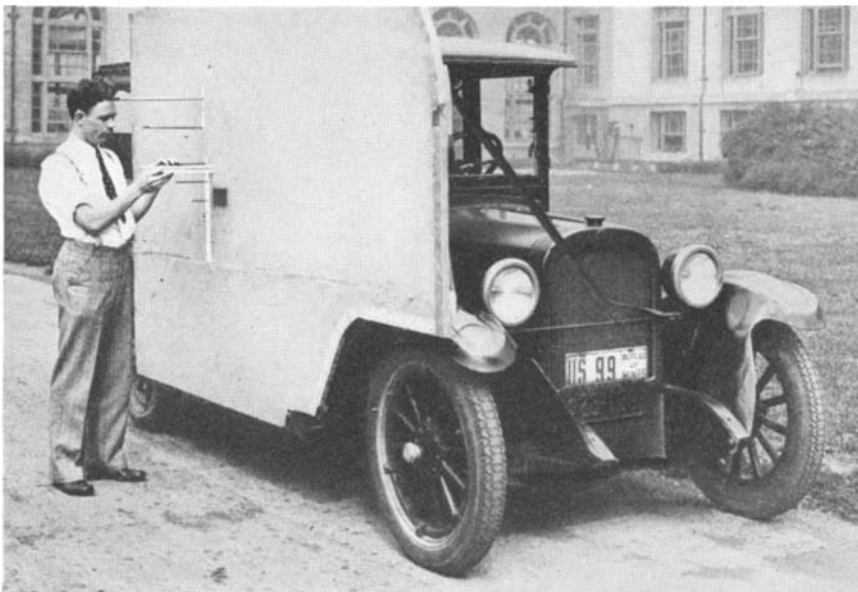
Studying effect of wind on heat losses from buildings. A wall section was set up on moving truck and Pitot tubes measured wind velocities while running
