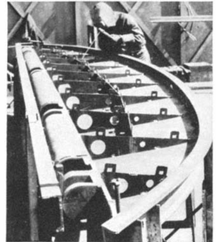
Ranger's rudder, four feet wide, was built up of arc-welded steel
