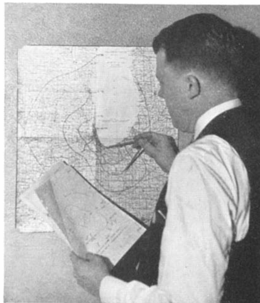
Checking the results of tests against the computed field pattern, which seldom varies more than a mile or so from that found in practice
