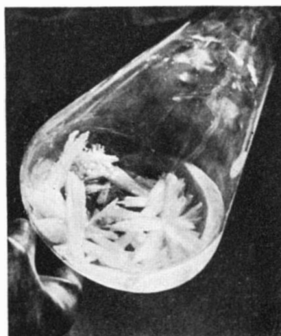
Radium-barium crystals produced during the final stages of the Curie fractional crystallization processes in the Eldorado refinery at Port Hope, Canada. In this flask is one gram of radium valued at 30,000 dollars. Radium is seldom reduced to metallic form: it oxidizes. It is left as a salt—usually sulfate
