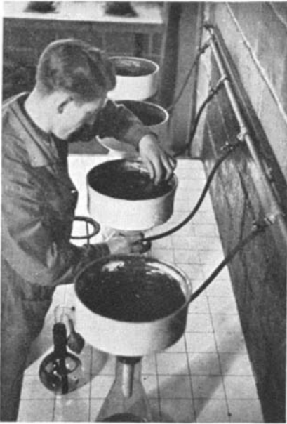
Filtering purified radium bromide at the Eldorado refinery before starting the evaporation of the barium content. The uranium, silver, manganese, and other by-product materials are separated during the earlier stages of the recovery
