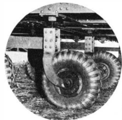
Close-up of the balloon truck tires and the leveling mechanism that makes it possible for the weight of the stage to be evenly distributed on its 224 tires
