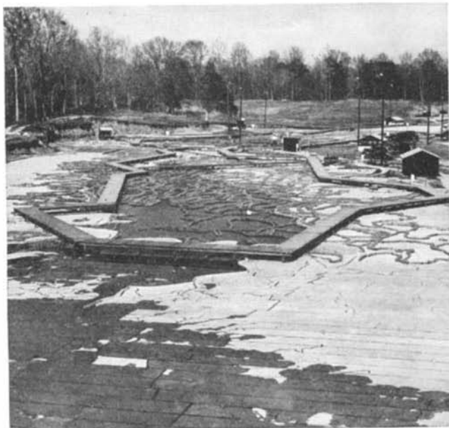
Below: The Atchafalaya Basin, looking north, with the Gulf of Mexico in the foreground. This model provides the engineers with data regarding the routing of rushing flood waters through the basin
