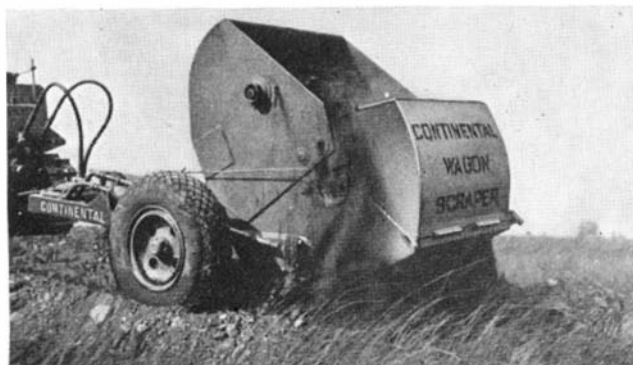
Hauling a load in the new four-yard scraper, and dumping it
