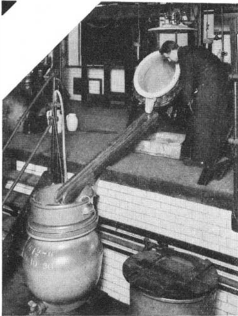
Platinum solution being poured from the dissolver via trough into the filter top
