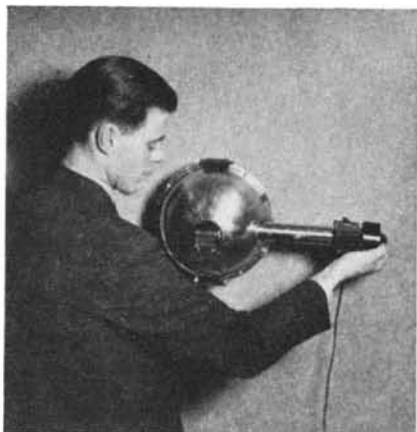
Determining the reflecting factor of a surface with the Reflectometer
