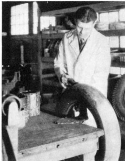
Stages in the process of retreading an automobile tire. Left: Inspecting the carcass. Upper left: Buffing off the old tread down to the fabric. Above: Applying cement to the casing. Upper right: Putting on the Camelback or new rubber tread. Right: Rolling the Camelback to expel air and insure all-over bond. Below: Removing the rebuilt tire from the circular retreading mold
