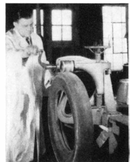
Stages in the process of retreading an automobile tire. Left: Inspecting the carcass. Upper left: Buffing off the old tread down to the fabric. Above: Applying cement to the casing. Upper right: Putting on the Camelback or new rubber tread. Right: Rolling the Camelback to expel air and insure all-over bond. Below: Removing the rebuilt tire from the circular retreading mold
