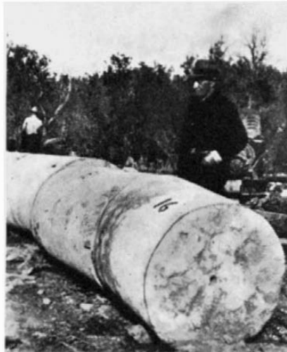
Drill core from a 36-inch hole
