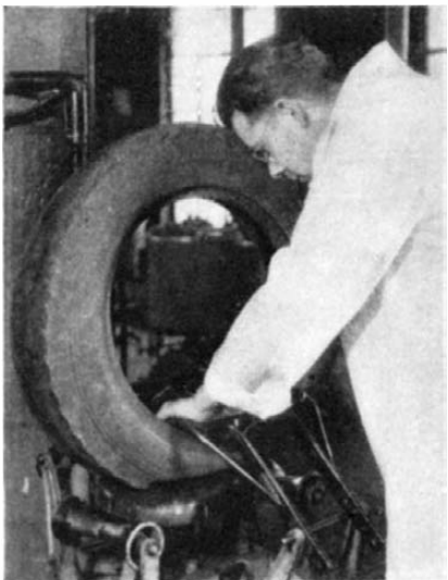
Stages in the process of retreading an automobile tire. Left: Inspecting the carcass. Upper left: Buffing off the old tread down to the fabric. Above: Applying cement to the casing. Upper right: Putting on the Camelback or new rubber tread. Right: Rolling the Camelback to expel air and insure all-over bond. Below: Removing the rebuilt tire from the circular retreading mold
