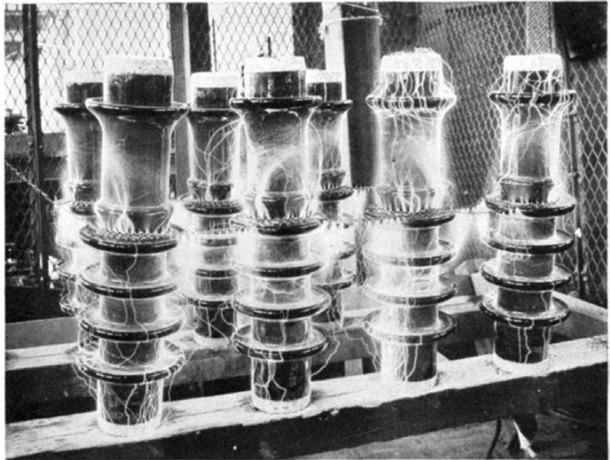
A literal bath of electrical fire surrounds these porcelain bushings on test at the Derry, Pennsylvania, Works of the Westinghouse Electric and Manufacturing Company. Flash-over takes place at 200,000 volts, the test being made to insure efficient service of bushings and insulators in high-voltage transmission systems
