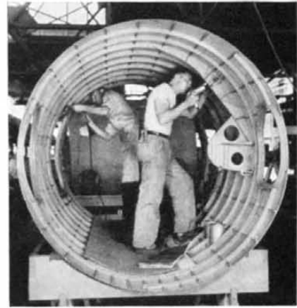
Riveting up the aluminum frames of one of the huge engine nacelles
