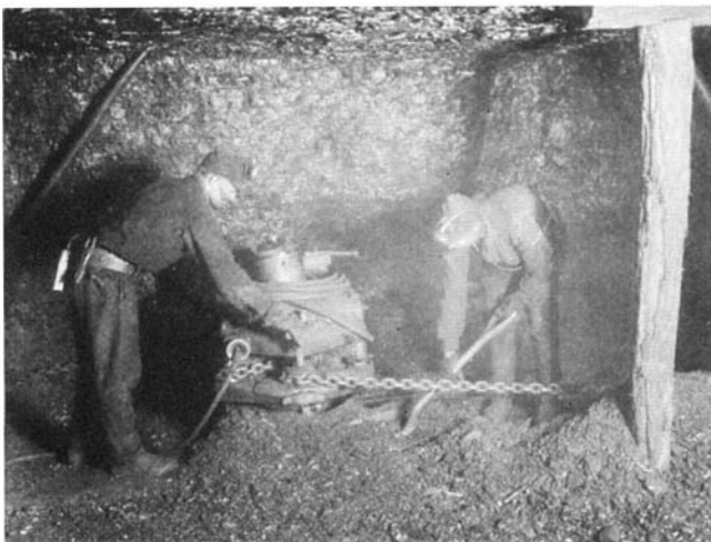
Coal mines constitute another dust hazard and especially at points where machines undercut the coal seam by means of powerful cutting teeth on a flat arm. At the right, this operation is rendered dustless by a spray of water on the cutting arm
