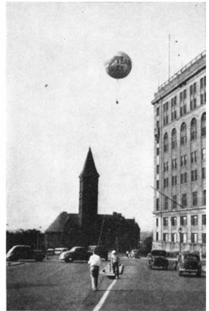
Above: Aerial camera and balloon in operation; guy ropes held by nearest man and one just visible in distance. Milwaukee Journal photo
