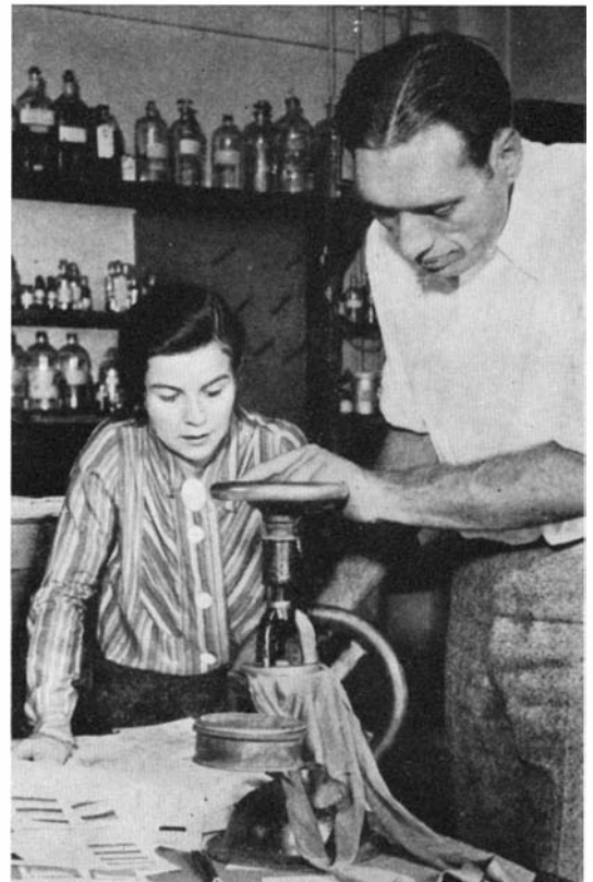
Manner in which the bursting strength of hoisery is determined in the Mellon laboratories
