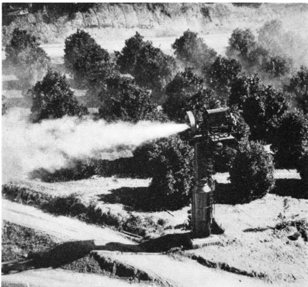
Although in actual use the heating machines give forth no smoke, smoke was added to the warm air to illustrate in photographs how the machine distributes heat over a
