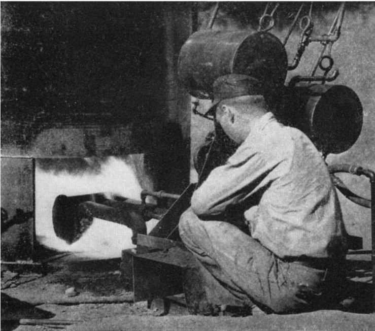
Oil burner at base of wind tower. Crude-oil flames impinge on a heat chamber, heat rises up the stack and is blown out over the fruit grove
