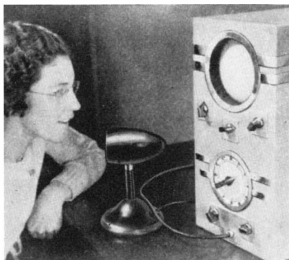
Left: A singer testing the pitch of her voice by watching the wave form on the cathode-ray tube screen. Above: The tuning forks and driving solenoids in the resonoscope
