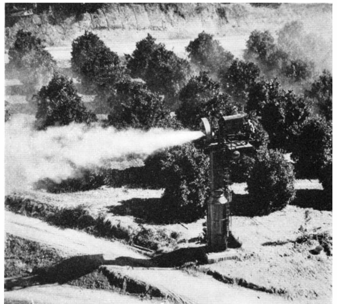
wide area. An automobile engine drives a six-bladed propeller and rotates the tower top. It is claimed that one of these machines can protect 10 acres of trees against frost
