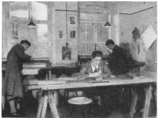
Photo-engraved rolls are inspected in foreground and "tooled" near windows to clean up and to correct errors
