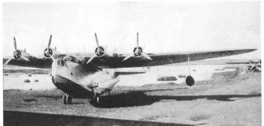
Not an amphibian, the XPBS-1 carries a beaching gear on board
