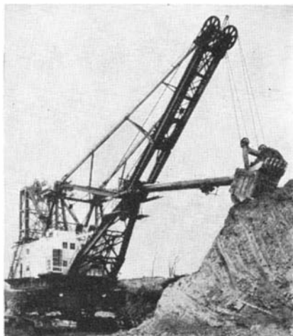
An electrical sense of balance keeps this 33-yard shovel on a level keel
