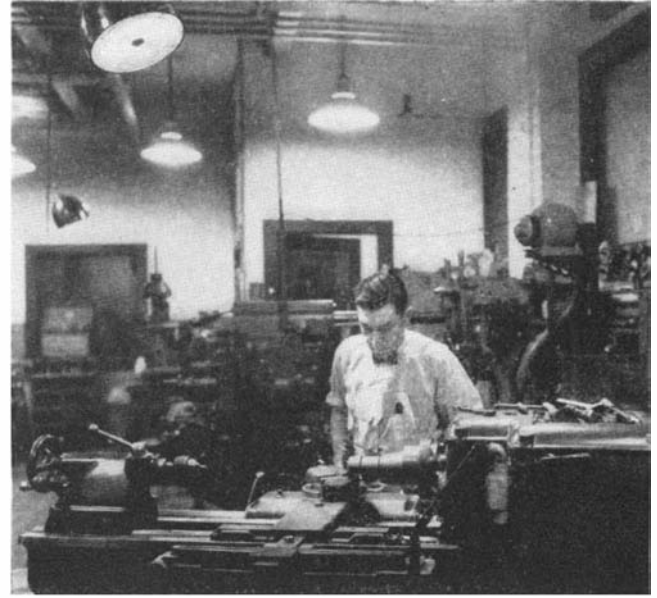
Striking difference between local, or spot, and general lighting of work. Contrasts are so severe in the scene at left that seeing is hindered rather than helped by the single bright light. The vast improvement with general lighting is shown at right
