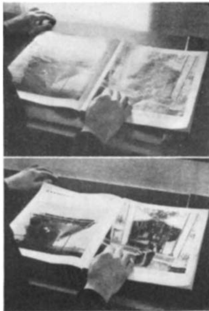
Ordinary lighting of a magazine (top) and resulting glare. Bottom: Same, lighted with polarized light
