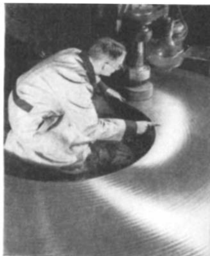
Smoothing the running surface of the world's largest thrust bearing
