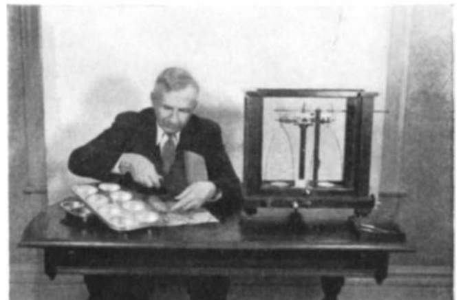
Sections of celluloid, cut from map tracings and weighed, determine crop or woodland acreages
