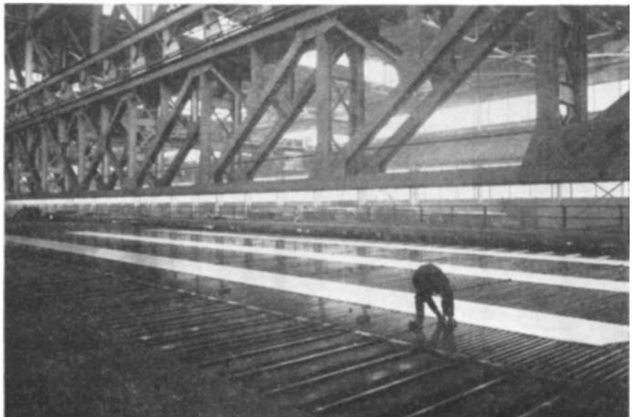
Steel is gaged on this transfer table on its way to finishing
