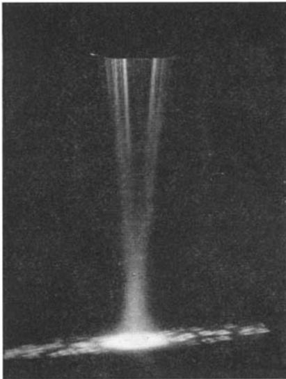
Above: How the new dental light focuses its rays to a concentrated beam. Below: A heat filter is between the light and the reflector
