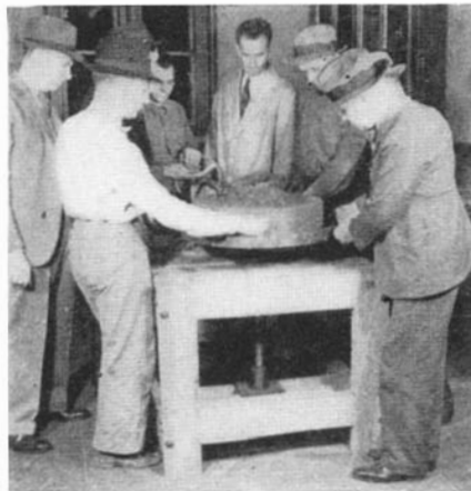
Members of the Louisville Astronomical Society edging a 20-inch disk of Pyrex on their machine in quarters lent by the University of Louisville, Louisville, Kentucky. In the group are a gas chemist, a garage owner, a manual training instructor, a paint maker, a mathematics professor, a type-caster, a bridge engineer, and the treasurer of a glass company—typical combination of amateurs. The society meets weekly, discusses astronomy and telescopes, and will ultimately complete this telescope of 100-inch focal length which will then be used jointly by the University, the public, and the makers
