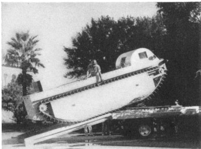
The mechanical "Alligator" is as much at home on land as in the water. It was designed for rescue work
