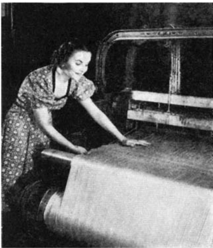
10 From marbles to cloth is a story of applied science opening a whole new field for an old-new product. The soft, satiny, pure-glass fabric shown below illustrates the possibilities. Present applications, however, are largely industrial rather than domestic; glass clothes, for example, are still in the future
