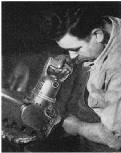
Electrically driven, these portable metal shears have many applications
