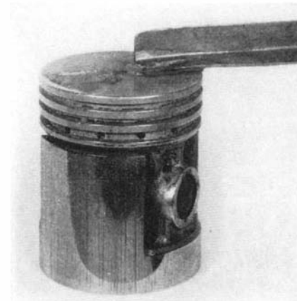
Soldering to chromium plated on aluminum to show tenacity of bond
