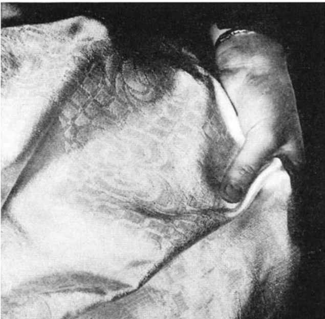
10 From marbles to cloth is a story of applied science opening a whole new field for an old-new product. The soft, satiny, pure-glass fabric shown below illustrates the possibilities. Present applications, however, are largely industrial rather than domestic; glass clothes, for example, are still in the future
