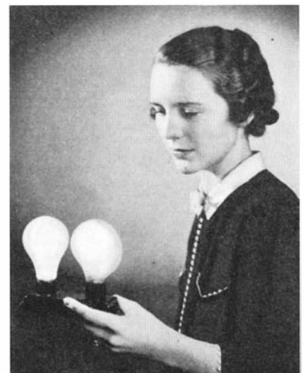
An incandescent lamp, subjected to intense heat in a building fire, bulged but remained burning. It is here compared with a standard bulb
