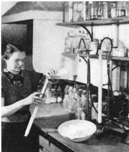
Left: Coating the inner walls of a new lumiline lamp. The fluorescent powder in solution is poured in; the excess is poured out. Above: A set-up of five of the new lamps
