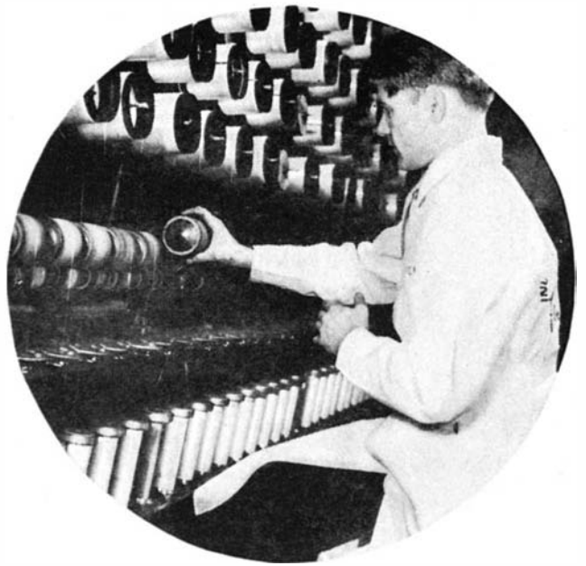
7 Whether continuous filament or staple fiber, the textile glass is now transferred to twisting equipment. Here two 102-filament strands are combined to form a single thread. Four strands so twisted are about the size of No. 50 cotton thread
