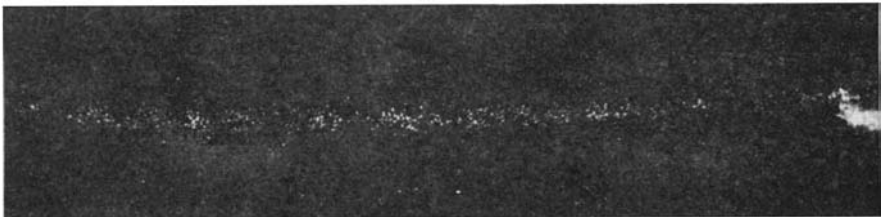
The trail of a normal cosmic ray electron, photographed by Corson and Brode under exactly the same conditions as the one above. Note how much less densely ionized the track is, compared with that left by the heavier particle
